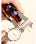
Your Patriot clutch spring heights have been preset at the factory and should require minimal adjustment. That measurement is taken from the top of the aluminum spring cap to the bottom of the red lever plate and is set at .675".
