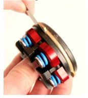
The clutch airgap is the space between the disk and the clutch pressure plate. The airgap is set at .015-.018" from the factory. The airgap is easy to check with a set of feeler gauges. Try different thickness feeler gauges until the feeler gauge will just snuggly fit between the top of the friction disk and the pressure plate.
