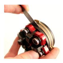
The clutch airgap is the space from the top of the floater and disk stack to the bottom of the pressure plate. The airgap is set at . 022-.026" from the factory. The airgap is easy to check with a set of feeler gauges. Try different thickness feeler gauges until the feeler gauge will just snuggly fit between the top of the friction disk and the pressure plate.
