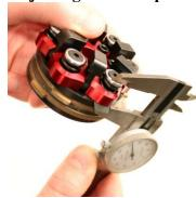
Your Patriot clutch spring heights have been preset at the factory and should require minimal adjustment. That measurement is taken from the top of the aluminum spring cap to the bottom of the red lever plate and is set at .650".
