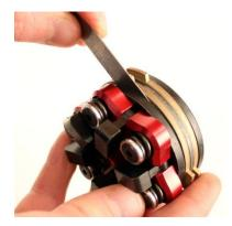
The clutch airgap is the space from the top of the floater and disk stack to the bottom of the pressure plate. The airgap is set at .022-.026" from the factory. The airgap is easy to check with a set of feeler gauges. Try different thickness feeler gauges until the feeler gauge will just snuggly fit between the top of the friction disk and the pressure plate.
